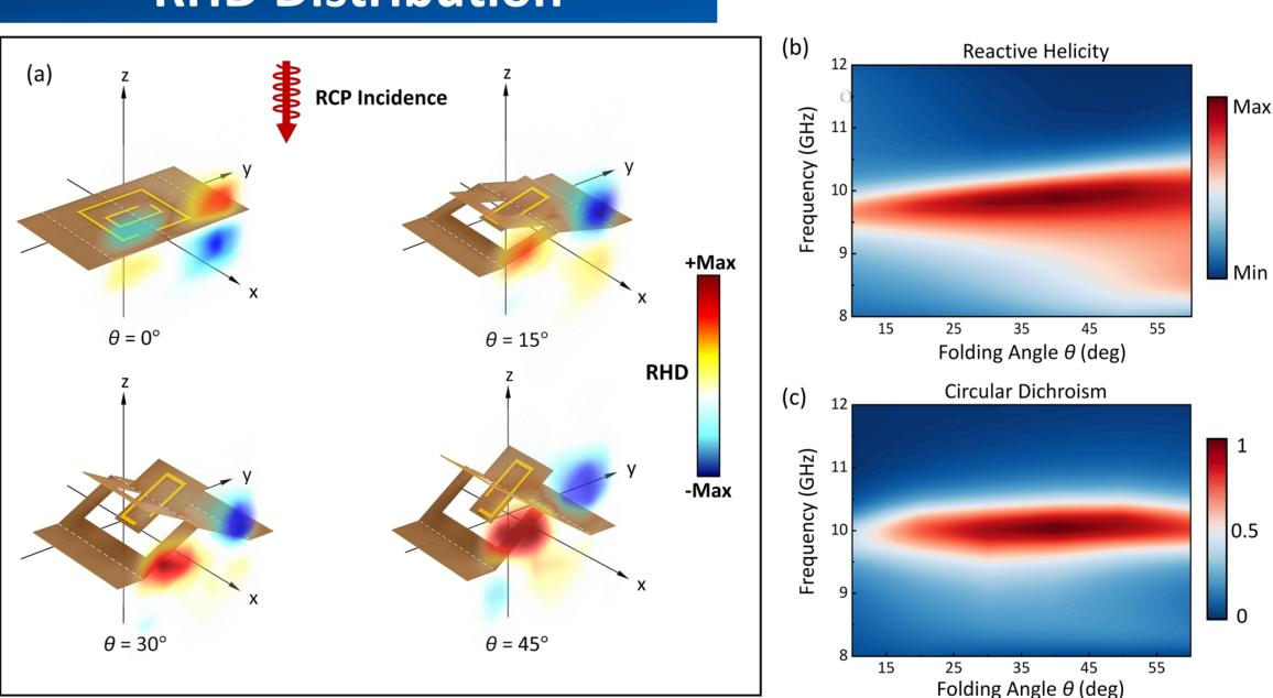
We introduce the Reactive helicity density (RHD) [4] as an evaluation metric, which plays a significant role in characterizing the generation of chiral radiation.
