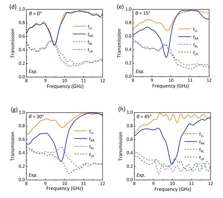
◆ The measured CD spectra calculated from (d)-(h) with peak value reaching 0.90 near 10 GHz.
